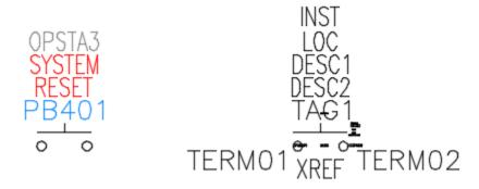
Additionally, AutoCAD<sup>®</sup> Electrical communicates through wires. This means lines in ACE are not just lines. ACE looks at them like actual wires, connected to the smart blocks. For example: if you have a layer called RED\_18AWG you would identify this as a wire layer. Wire numbers could be assigned to lines on this layer and reports could be generated.
