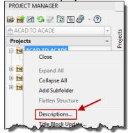
The AutoCAD<sup>®</sup> Electrical project information is currently empty, but that will be changed shortly. The names for each line, such as Line1, Line2, etc, will also be changed to be better description labels. *Note: The check mark for "in reports" means the data on that line is available for use in reports such as Bills of Materials. It doesn't affect the title block.*
