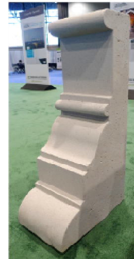
Figure 8. Precast cornice cast by Gate Precast using the prototype 12-inch deep cornice mold.
