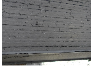
Printing pattern that decreases underfilling and voids
