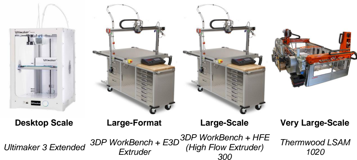
Figure 3: Differences in terminology describing scale of 3D Printers.
