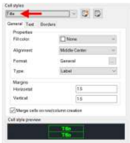
Fig.34 – This shows the cell style settings for the Title cell in the new table style
