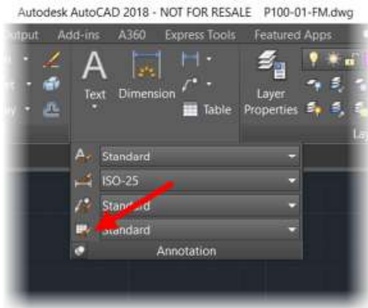
Fig.30 – The Table Style icon on the flyout menu on the Annotation panel on the Home tab on the ribbon
