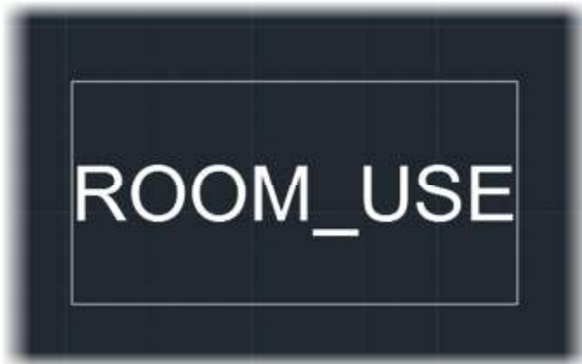
Fig.28 – A rectangle and a room use attribute on layer 0, ready to be made in to a block
