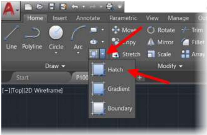
Fig.9 – The HATCH command on the Draw panel on the Home tab on the ribbon
