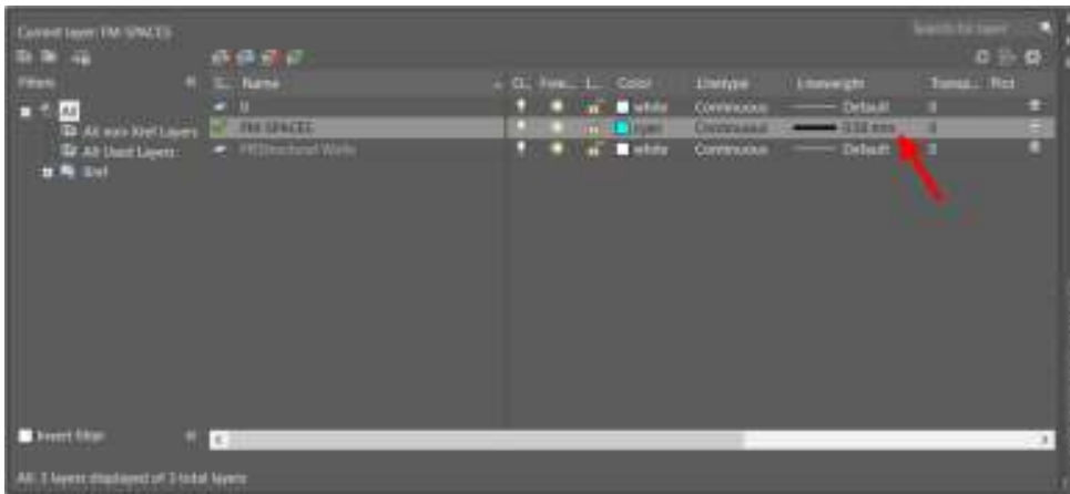
Fig.17 – The Layer Properties Manager showing that the FM-SPACES layer has a lineweight applied to it
