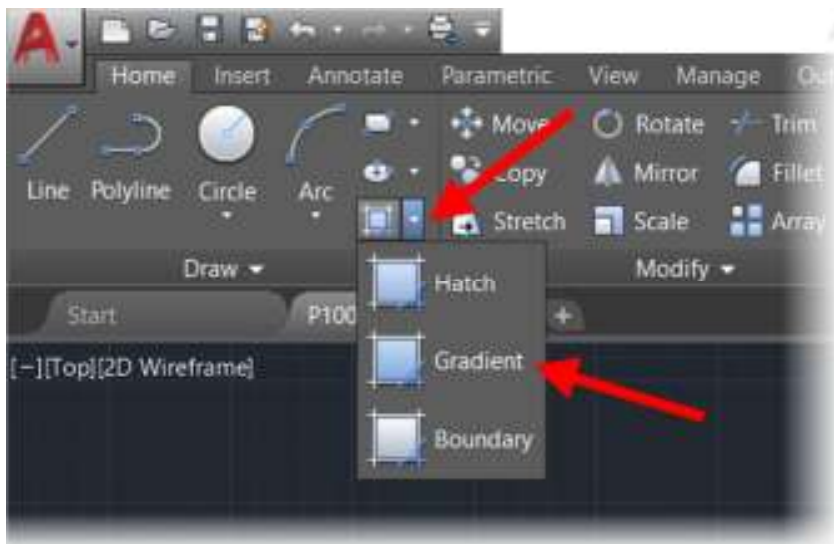
Fig.7 – The GRADIENT command on the Draw panel on the Home tab on the ribbon
