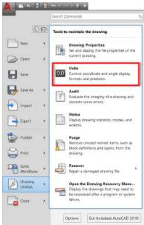
Fig.5 – The Application Menu displaying the Drawing Utilities section with the UNITS command highlighted
