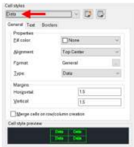
Fig.36 – This shows the cell style settings for the Data cells in the new table style
