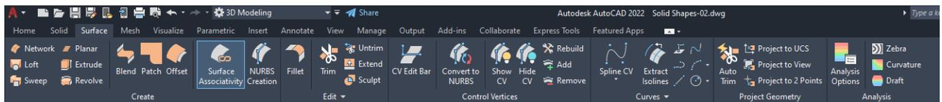
3D Surface creation tools are similar to the 3D Solid tools such as sweeping, lofting, extruding, and revolving. 3D Surfaces can also be created by blending, patching, offsetting, filleting, and extending other surfaces. They do not contain volume/mass properties.
