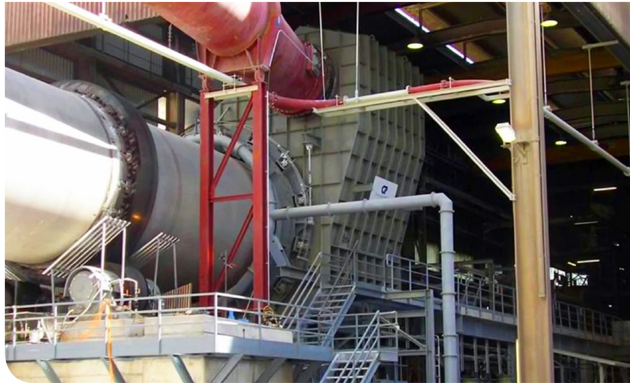
The ETA Cooler at the Holcim Untervaz Cement Plant in Switzerland is a huge machine that’s almost half a football field in size. Courtesy of Claudius Peters.
