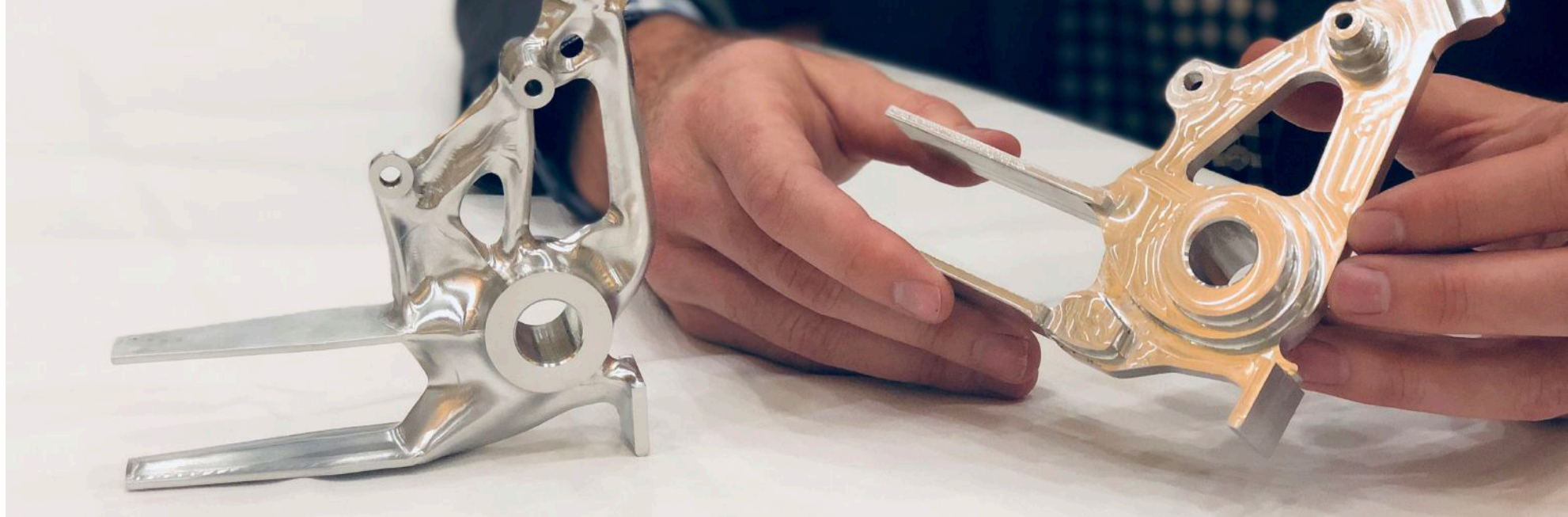
Both of these parts, produced by generative design, feature traditional CNC milling techniques: 3-axis (left) and 2.5-axis.
