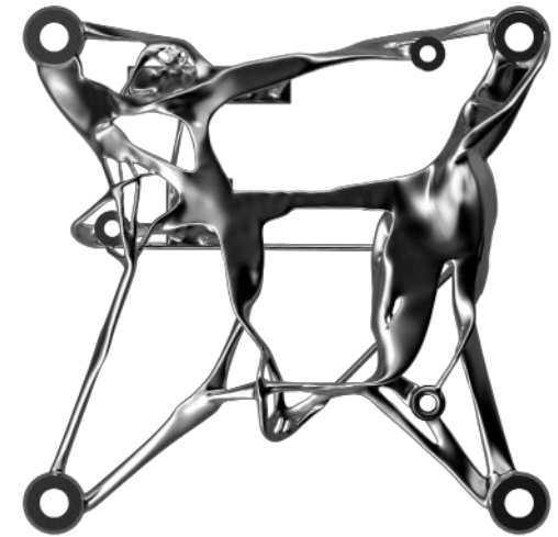
Another view of the initial ECU frame, made using generative design. Courtesy of DENSO Corporation.
