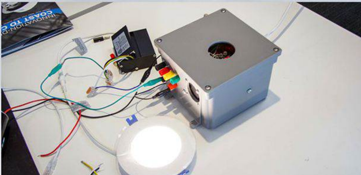
This black box will allow off-the-shelf, low-voltage devices to be powered by Ethernet and talk to other devices. Courtesy of WZMH.
