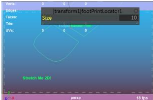
Figure 18: Snapshot shows the footprint manipulator. The “Stretch Me!” and “Stretch Me 2D!” UI are drawn using MUIDrawManager for the manip. The in-view editor is drawn for the plug-in internally. Note that it is layered to be on top of the footprint plug-in and spReticle UI, as well as the internal UI (polygon statistics shown here as an example).
