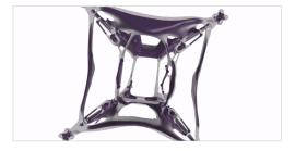
Consider designing a chair. Instead of drawing two, three or even 10 options, you can tell the computer you want a chair that supports 110kg weight, costs \$30 per unit, and uses 12kg material. The computer, using cloud computing to increase processing power, can then deliver hundreds of practical and manufacturable design options that all meet those criteria.
